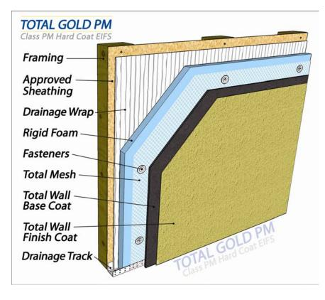
The **Total Gold PM** system is a class PM Hard Coat EIFS which uses Extruded Polystyrene (XPS) rigid insulation boards and can be installed over virtually any substrate.
