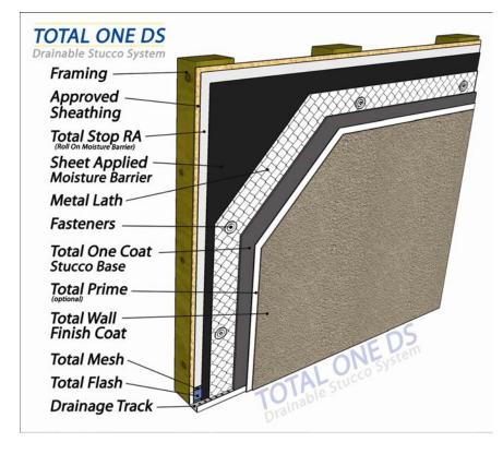
The **Total One DS** system is a premium drainable hard coat stucco system. It is designed for maximum performance and weather protection and is backed by an extended warranty.
