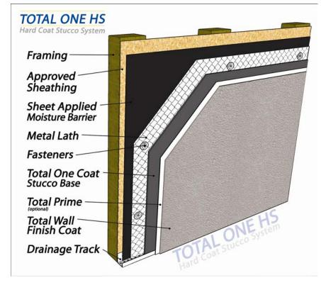
The **Total One HS** system is a traditional hard coat Portland cement stucco that can be used over virtually any substrate.
