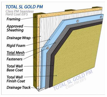
The **Total SL Gold PM** system is a seamless Hard Coat Class PM system without the need for control joints for spans under 50 lineal feet and is applied over virtually any substrate.
